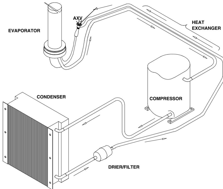
FIGURE 3. Typical refrigerant circuit
