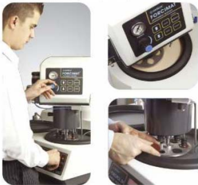
By using the FORCIMAT automatic head, the efficiency increases and same consistent sample quality is guaranteed
