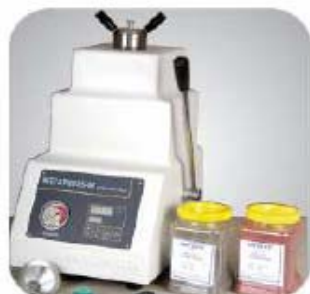
Setting and display of mounting parameters digitally ensures reproducible results.
