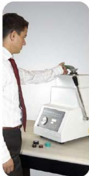
Setting and display of mounting parameters digitally ensures reproducible results.
