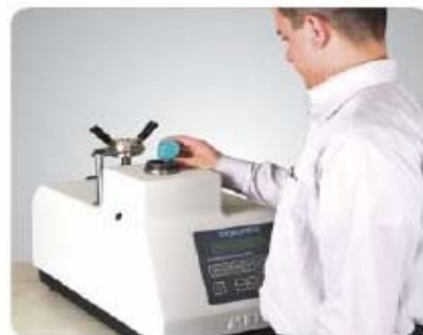
Electro-hydraulic pump and preprogrammed moulding sequences allow a smooth and comfortable operation.
