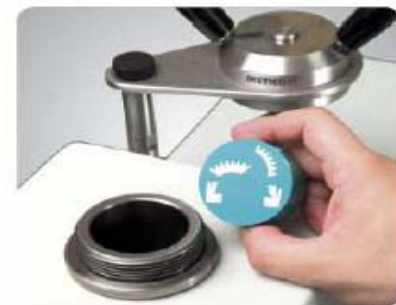
Electro-hydraulic pump and preprogrammed moulding sequences allow a smooth and comfortable operation.
