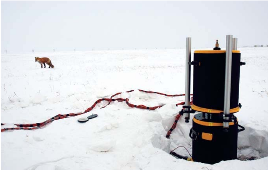
A10 deployed from a Sno-Cat in the Arctic (-40°C. Note these extreme conditions require slight modifications to the standard instrument configuration).
