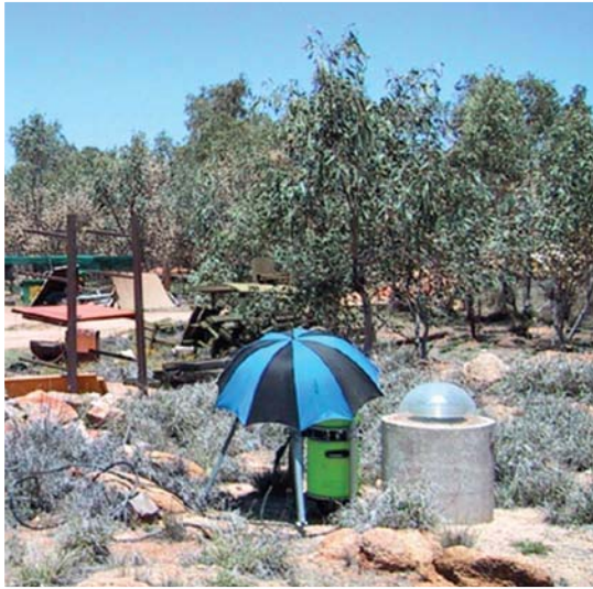
A10 deployed from a light vehicle in Australia (+40°C. Note these extreme conditions require slight modifications to the standard instrument configuration)
