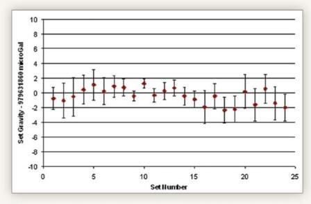
Shown above are the results of a 24-hour site occupation (24 sets of 100 drops each). The set scatter is on the order of 1  $\mu$ Gal, indicating sub- $\mu$ Gal measurement precision.
