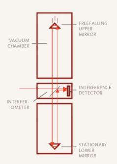
Mesures) proclaimed the ballistic freefall method as an official primary method for measuring gravity.
