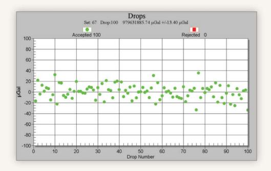
Shown above are typical gravity measurements. Note final precision after 2 minutes is approximately  $2\mu\text{Gal}.$
