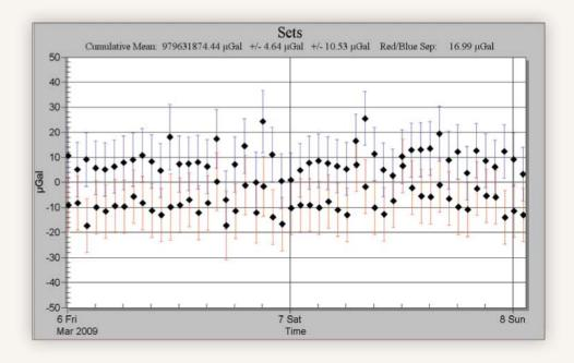
Shown above are typical gravity vales for sets of 100 measurements. The final precision is less than 2  $\mu$ Gal.
