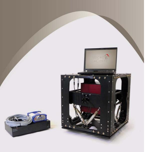
Smaller sensor, full feedback system, and a host of other features takes the world's best dynamic gravity sensing system to the next level.
