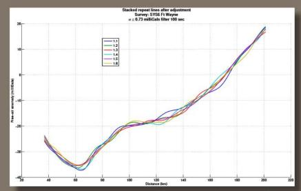
Shown above are six repeat measurements of the free-air anomaly acquired on a flight line near Fort Wayne, Indiana. With a 100 second filter, the standard deviation of the repeats was 0.73 milliGal. Note that during the acquisition of Line 1.1, the aircraft encountered a large wake turbulence event (figure below) which produced no measurable effect in the processed gravity.
