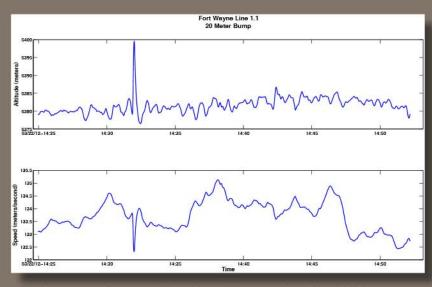
Altitude (meters) and speed (meters/second) of the aircraft for Line 1.1 in the above figure. Horizontal axis is GMT time. Note that the large vertical acceleration experienced by the aircraft is not reflected in the resultant gravity measurement.
