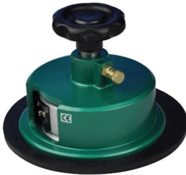
**SUAJE DE CORTE MODELO TF513A MARCA TESTEX, PARA MUESTRAS MANUAL.**
